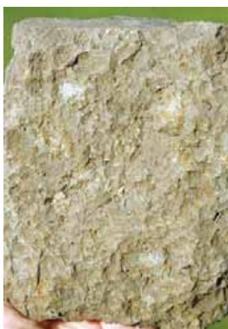
MODERATE CONDITION VS = 1 Soil has many (10–20 percent) fine and medium orange and grey mottles.
